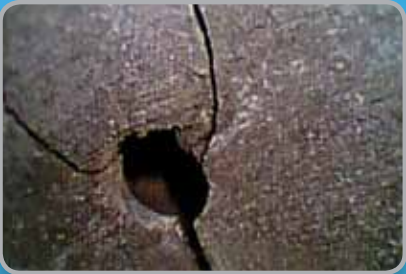
Using the Close-Focus tip, fine cracks are detected inside a combustion chamber.
